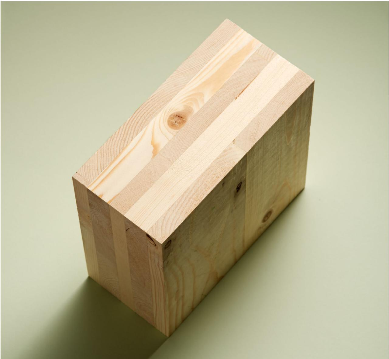
**Cross laminated timber is a form-strong and lightweight building material that is used as frame in modern high-rise buildings.**
